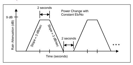
The minimum specifications of the Rain Fade Simulator are:
